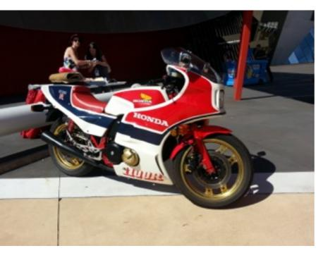
the first model. Much strengthened wheels, the front an 18 rather than 19 inch, were added, and the suspension also significantly overhauled. changes were made to enhance engine reliability, notable the cam chain and tensioner. Front discs were also now ventilated. original red on white paint scheme was retained but the seat and fairing now added Honda royal blue as well. Just as gorgeous, and more effective, was the Another timeless classic. verdict. Some 1500 RCs were built in all.
